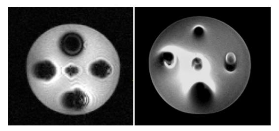
Figure S1. The five ENDS imaged with a gradient-echo sequence (left) shows characteristic dipole pattern disturbances from the different magnetic field susceptibilities found in the materials used to construct the varied ENDS. The same phantom images with a spin-echo sequence (right) removes the susceptibility-induced distortion and signal loss, but the RF field is compromised by the presence of conductors.
