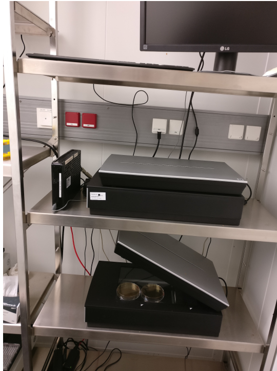
Appendix 0 Figure 10. Image of the scanner system. Photograph of the scanner system used for time-lapse imaging of phage spread in spatially structured bacterial populations. Three scanners (Epson Perfection V600 Photo Scanner) simultaneously scanned 12 plates in total every 20 minutes in 30°C for 48 hours per experiment.
