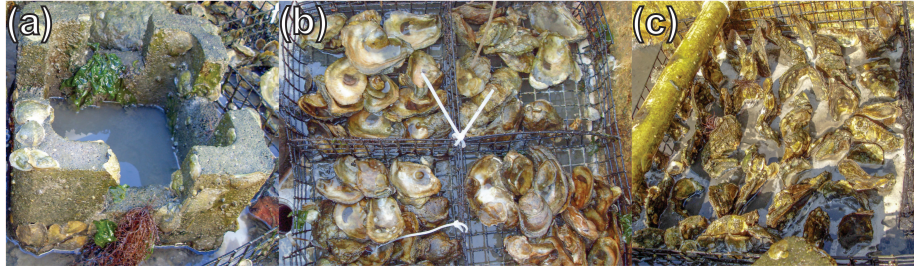
Figure 1: Photographs of the experimental reef substrates utilized in the mesocosm and field experiments, including (a) Oyster Castle®, (b) unconsolidated oyster shell, and (c) oyster shell embedded vertically in concrete.
