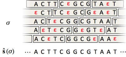
Fig. 3. Part of a consistent assembly for L = 5 and D = 2 . Notice that there can be at most D erasures per read and per “column” of the assembly \sigma . Moreover, all non-erased bases in a column must agree.
