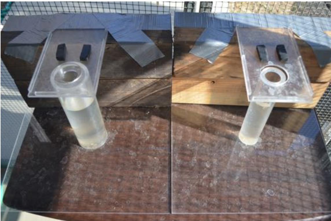
279 Figure 6. The Narrow vs. Wide with equal water levels experimental set up.
