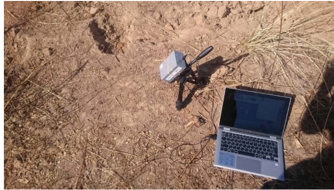
Photo 2. The compact hyperspectral sensor with a USB camera. The camera was set up at a right angle from the sun to avoid the shadow.
