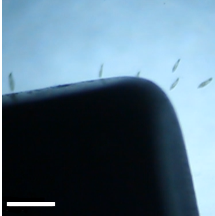
Fig 2. Photomicrograph showing magnetite nanoparticle-treated P. caudatum being drawn to a magnet. Scale bar = 500 \mu\text{m} .
