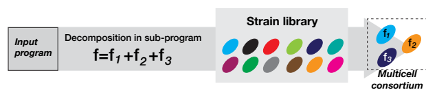
Figure 1. Distribution of logic programs within a multicellular consortia. The logic program of interest (either Boolean logic or history-dependent program) is decomposed as a disjunction (=sum) of sub-programs. A given function f encoding the program behavior is decomposed into functions f_1 , f_2 and f_3 encoding sub-programs. 3 strains performing f_1 , f_2 and f_3 are selected from the strain library to assemble a multicellular consortia computing the desired program.
