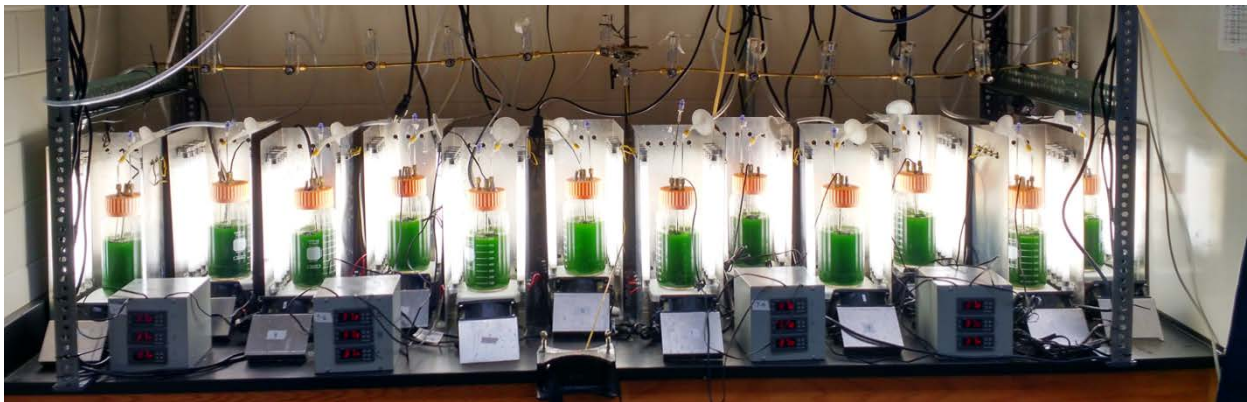
Figure 1. Photobioreactor System in Operation. This 12-reactor system was used to simultaneously grow cyanobacteria under varying conditions. Gas delivery could have the same composition for all 12 reactors or one composition for the first six (from the left) and a different composition for the second six. Temperature control systems were combined in sets of three, but temperature set points were independent for each reactor.
