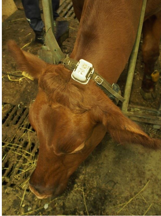
Figure 1. Ubisense tag attached to the collar of the cow.
