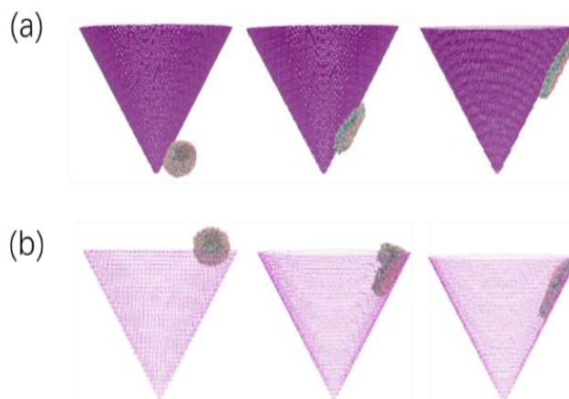
Fig 4. The rupture of vesicles on (a) outer surface and (b) inner surface of a conical surface.
