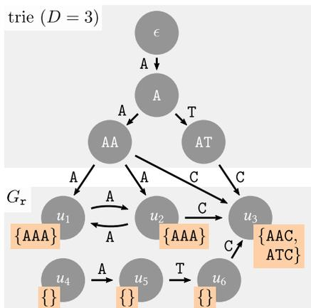
Fig. 3:  $G_{\mathbf{r}}^+$  enables semi-global alignment by extending  $G_{\mathbf{r}}$  with a trie.
