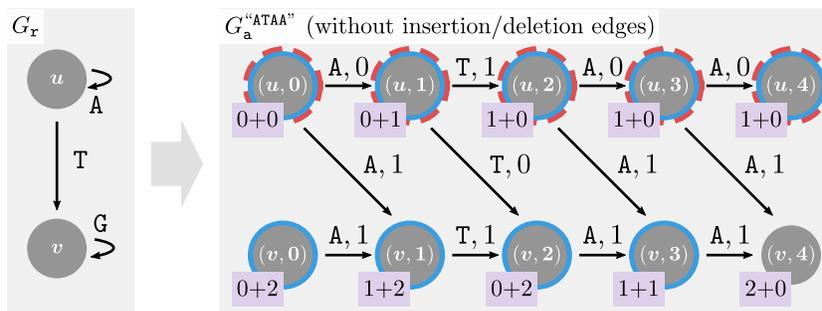
Fig. 2: The benefit of using our heuristic over DIJKSTRA. Alignment graph  $G_a^{\text{ATAA}}$  (right) is based on reference graph  $G_r$  (left), but omits insertion and deletion edges for simplicity. The pink boxes  $g+h$  indicate the distance from the sources  $S = \{(u, 0), (v, 0)\}$  (in  $g$ ) and the cost of aligning the next  $d = 2$  letters (in  $h$ ). DIJKSTRA (resp.  $A^*$ ) expands states circled in blue (resp. dashed red).
