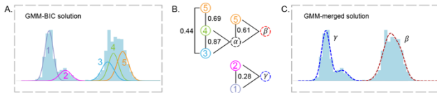
Figure 6. An example of merging Gaussian mixture components. A) Illustration of the 5 original Gaussian components in a 1-D GMM model. B) Merging components into component complexes. C) The final component complexes after merging. The dashed lines represent the density curves of the two merged component complexes \beta and \gamma .
