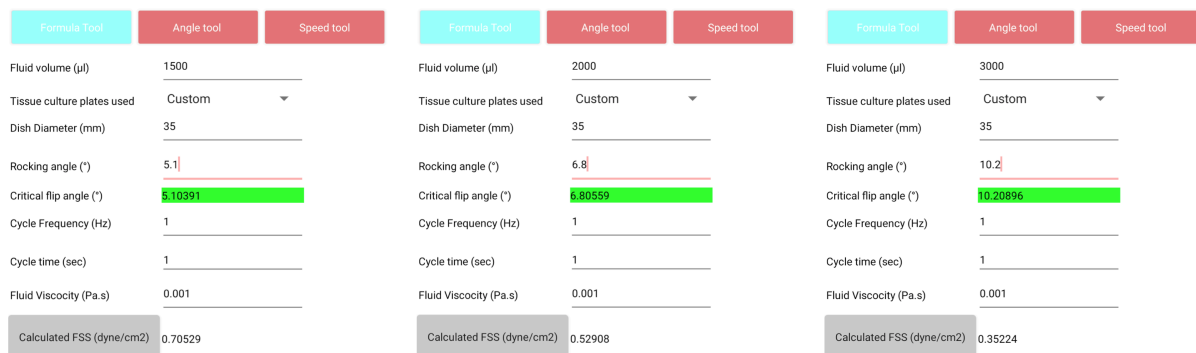
Figure 4. ShearFAST formula tool reproduces the example data reported in the supplementary data of the original publication original publication
