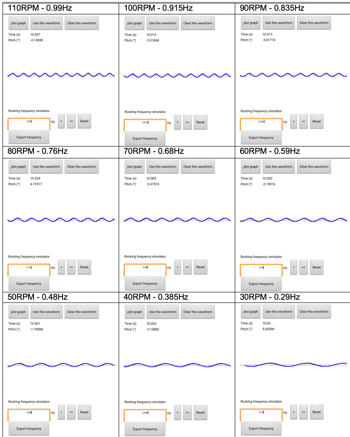
Figure 6. ShearFAST measured rocking frequencies at rocker defined rocking speeds (RPM). Illustrating the value of the ShearFAST approach; when manually selecting the rocking speed 60RPM (i.e. 1Hz) the resulting profile was visibly slower. ShearFAST determined a rocking speed of 0.59Hz which was corroborated by later video analysis (Table 1).
