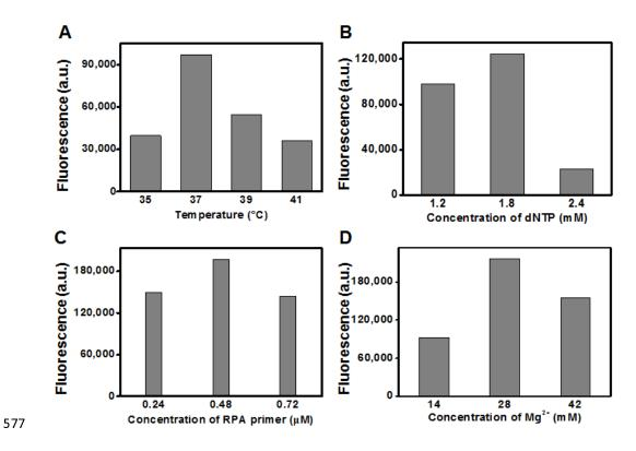
578 Figure 3. Optimization of MTBC-Cas12a trans-cleavage fluorescence assay.
