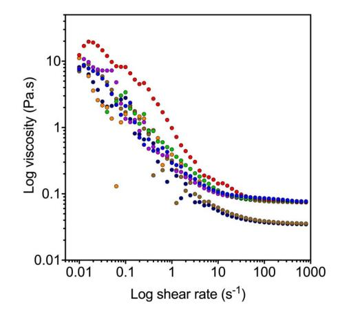
**Figure 4.** Multiple flow sweeps of 200 mg/mL (20 % w/v) N-R<sub>7</sub>-C. Each sample displayed shear thinning to near identical viscosity following repeated runs. Four repeated runs were carried out for two samples. Shear history did not appear to have an effect on the rheology of the sample.
