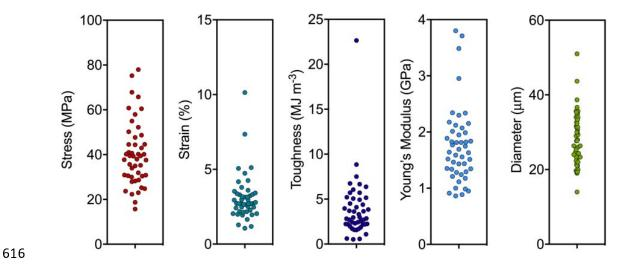
617 **Figure 8**. Mechanical testing of synthetic spider silk fibers from N-R<sub>7</sub>-C. Mechanical properties were
