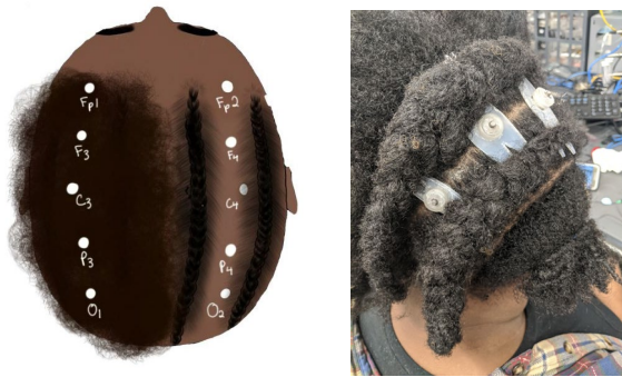
Fig. 4: Our experimental protocol setup: The right half of each participant’s hair was braided, while the left half remained unbraided. Every labeled point bore a gold cup electrode, while the braided points bore a Sevo electrode as well. (left) Schematic diagram of electrode placements; (right) Photograph of Sevo electrodes placed on a braided participant.
