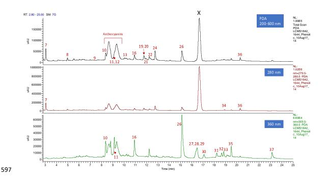
**Supplementary Figure 2.** Liquid Chromatography-Mass Spectrometry (LC-MS) chromatograms for BerriQi® concentrate, showing PDA (photodiode array) phenolic profiles measured at 200–600 nm, 280 nm and 360 nm. Peak numbers refer to compounds listed in Table 1. X, denotes sorbic acid, a preservative added to the BerriQi concentrate during formulation. This was present at a concentration of ~2000 µg/mL.
