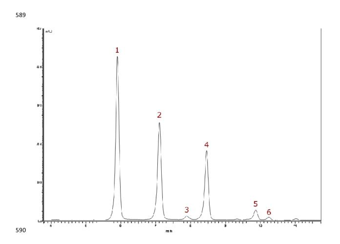
591 **Supplementary Figure 1.** Liquid Chromatography-Mass Spectrometry (LC-MS) 592 chromatogram for BerriQi® concentrate, showing the anthocyanin UV/VIS profile 593 measured at 520 nm. Peak numbers refer to compounds listed in Table 1.
