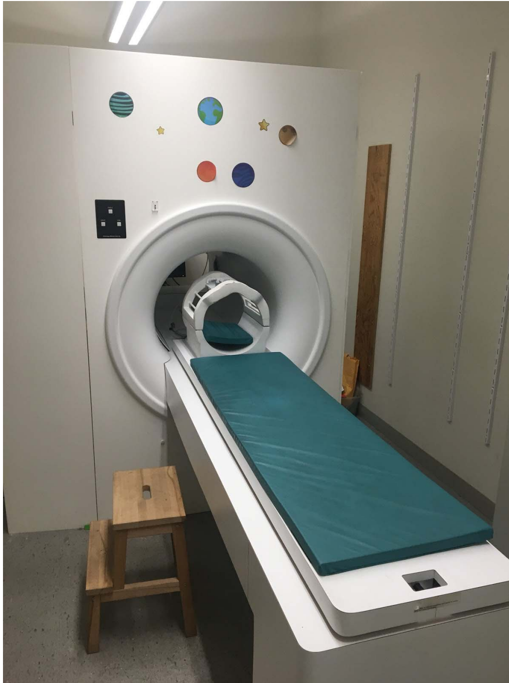
Fig. 1 The mock-scanner used in this study. A motorized bed is used to move the participant back into the bore. The participant views visual stimuli through the use of a mirror on the head-coil. The participant wears headphones to hear sounds from the movie. Speakers (not visible in the photo) are used to play gradient sounds while the participant lay in the mock-scanner
