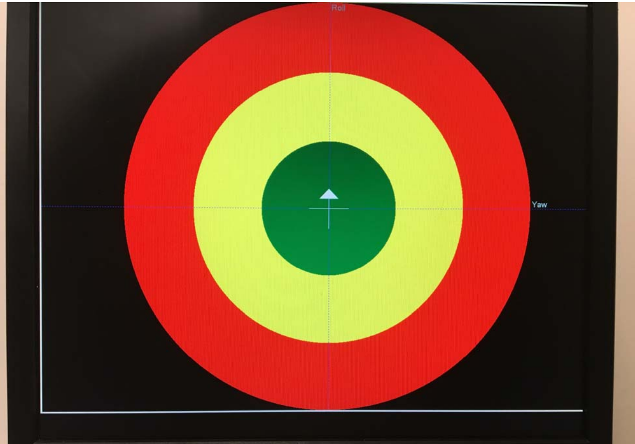
Fig. 2 The target system used in conjunction with MoTrak software. The cursor (shown in the center of the target as a cross) tracks participant head movement. This screen is visible to the participant at the back of the mock scanner through a mirror system. Head movement results in the cursor moving on the screen—hence, the participant can see how their movement causes the cursor to move. Participants are encouraged to stay in the green circle as much as possible. Depending on the step of the mock scan protocol (see below for more details), verbal feedback is also given to the participant (“You moved your arms, and it caused your head to move; did you see that on the screen?”)
