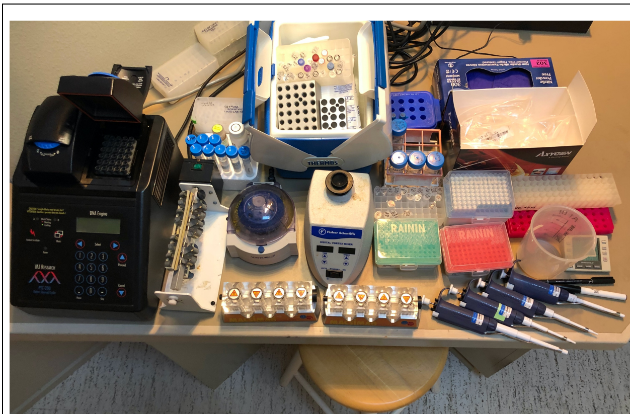
Figure 2: Equipment, supplies, reagents and solutions for CUT&Tag@home. Steps 1-8 for all experiments were performed on this counter in a home laundry/utility room using stock solutions and frozen nuclei aliquots previously prepared in the lab. There are no hazardous materials or dangerous equipment used in this protocol, however appropriate lab safety training is recommended.
