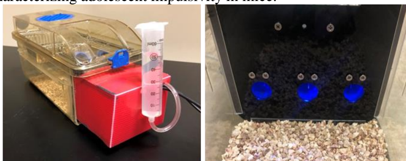
Figure 1. The DIY-NAMIC system is integrated into the homecage of standard mouse cages. The Arduino and all components of the DIY-NAMIC system are enclosed within the red encasing with the exception of a syringe for water or liquid reward, mounted on the outside (left). Modified cages remain compatible with most standard high-density ventilated racks. Inside homecage view of the DIY-NAMIC system including three nose ports with blue LEDs illuminated, each of which contain a spout for liquid reward (right).
