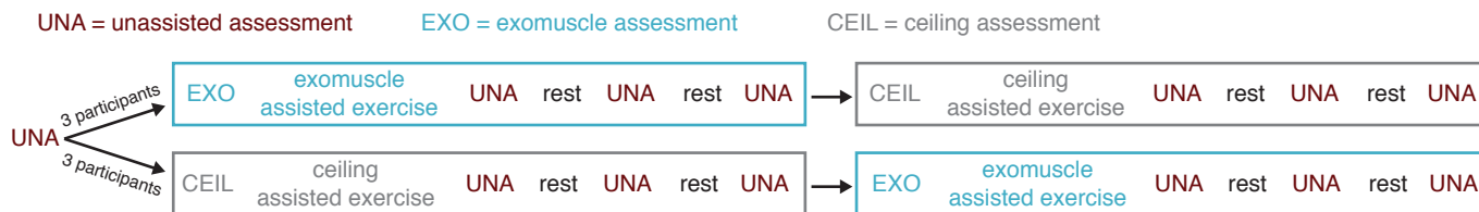
Fig. 5. Experimental protocol followed by stroke survivors. Participants performed a baseline assessment without support from either test device. Participants were then randomly assigned to use the exomuscle or ceiling support first. They performed an assessment with that support followed by a 10-minute supported exercise. Follow-up assessments punctuated by 10-minute rests were performed after each exercise to gauge residual effects of device use. Participants then repeated this set of tests with the other support. Each assessment consists of a workspace measurement and the recording of a proxy for flexor synergy activation.
