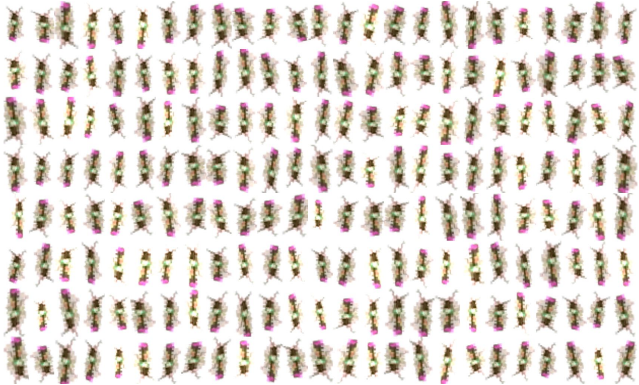
Appendix-figure 7: Dataset augmentation using TensorFlow's intrinsic mechanism for image transformation on a single example image to generate a larger training dataset.
