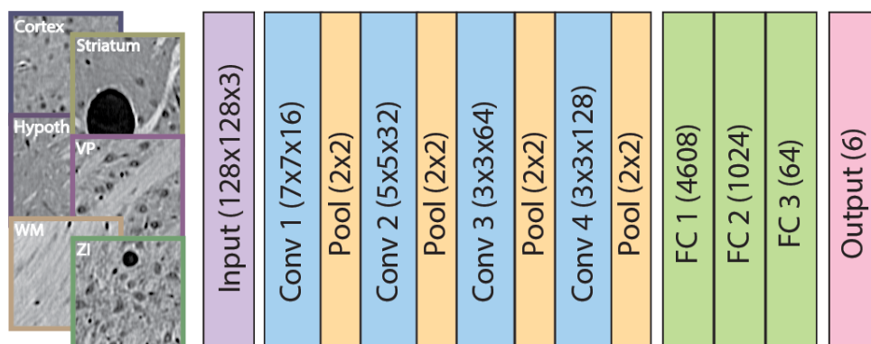
Figure S1: CNN architecture . The network used in our experiments is a 7-layer feed-forward deep convolutional neural network. The (k, k, c) convolutional layers (shown in blue) have c filters in the layer, each with a receptive field of size (k, k) . All the convolutional layers have stride = 1. The first two layers have padding = 1 while the last two convolutional layers don't use any padding. The pooling layers (shown in yellow) used throughout perform max pooling and have a stride of 2. The fully connected layers (shown in green) and each of them has d nodes in the layer.
