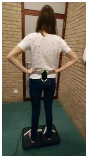
Figure 1: Test setup. Participants stood barefoot on the force plate (1 meter in front of the wall) in a comfortable posture, both hands positioned at hip level. The smartphone was attached to the participant's back at the level of the second sacral vertebra, near the body center of mass.
