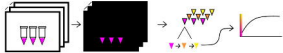
Figure A1. Masks are created by drawing polygons around the pixels representing the reaction. The masks are then applied to each frame, and the values of the isolated pixels are obtained and plotted against time.
