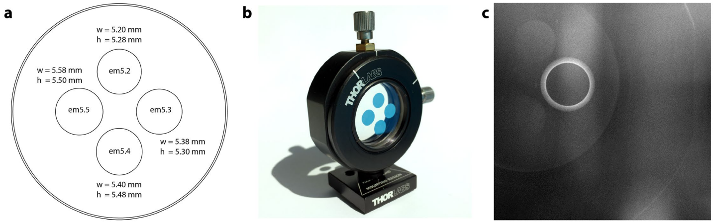
Supplementary Figure 3: Elliptical masks. a , Specification of the masks dimension, designed to be placed at an angle of 10^\circ in the beam path. b , Picture of the four elliptical masks deposited on the glass window and housed in a 2D translation mount. c , Camera image of the BFP with stray light highlighting the masks and the holder.
