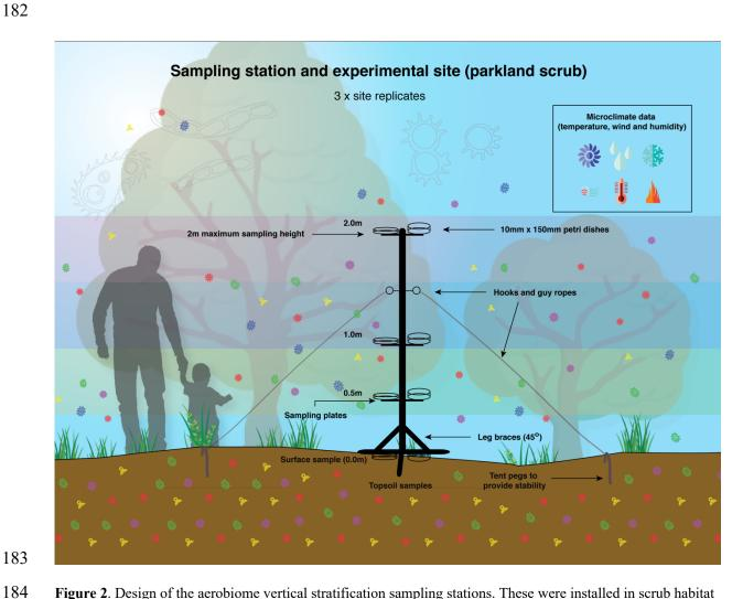
**Figure 2**. Design of the aerobiome vertical stratification sampling stations. These were installed in scrub habitat in the Adelaide Parklands.
