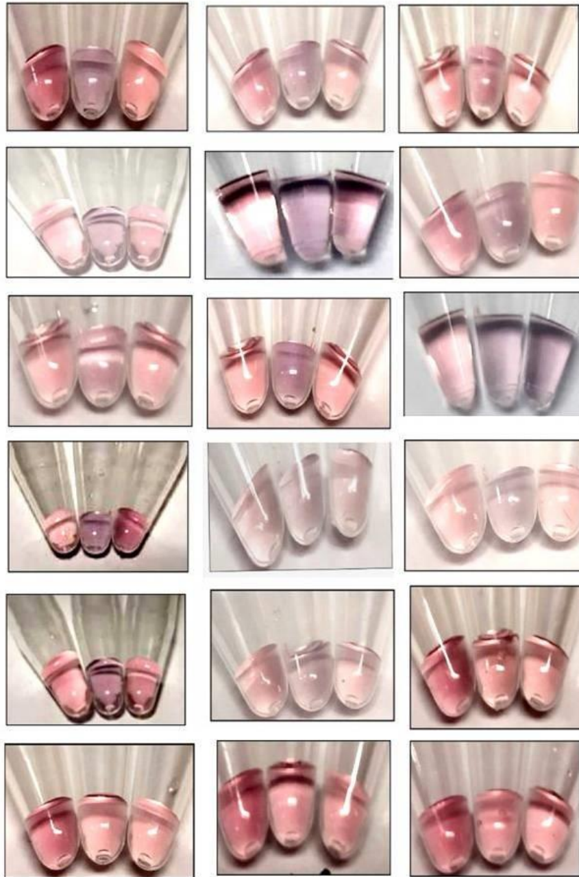
Figure S2. The figure shows optical images comparing assay performed with NTC (left vial), RNA from clinically diagnosed nCOVID infected subjects (middle vial), and RNA from subjects without nCOVID infection (right vial). Clinical diagnosis of the subjects based on Taqman RT-PCR analysis is given in Table S1
