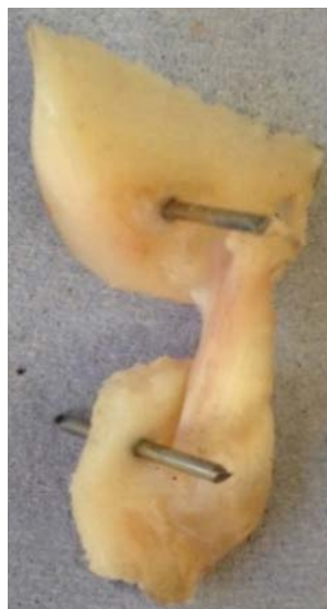
Figure 1: The extracted cranial cruciate ligaments (CCL) consisted of approximately 10 mm of the femoral and tibial bones forming femur-CCL-tibia complex. Two 1.1 mm arthrodesis wires were drilled through the bones to facilitate clamping of the sample.
