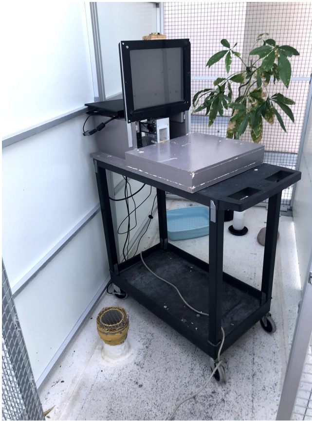
Figure 1. Touchscreen-equipped operant chamber basic set up during food hopper training. The computer monitor sits behind a touchscreen panel, and food is delivered via a food hopper that is moved by a robotic arm. The programs are run on a laptop located at the back of the touchscreen, and the laptop can be remotely controlled from outside the aviary using the experimenter's laptop. Unlike most TOCs, our setup is not an enclosed chamber.
