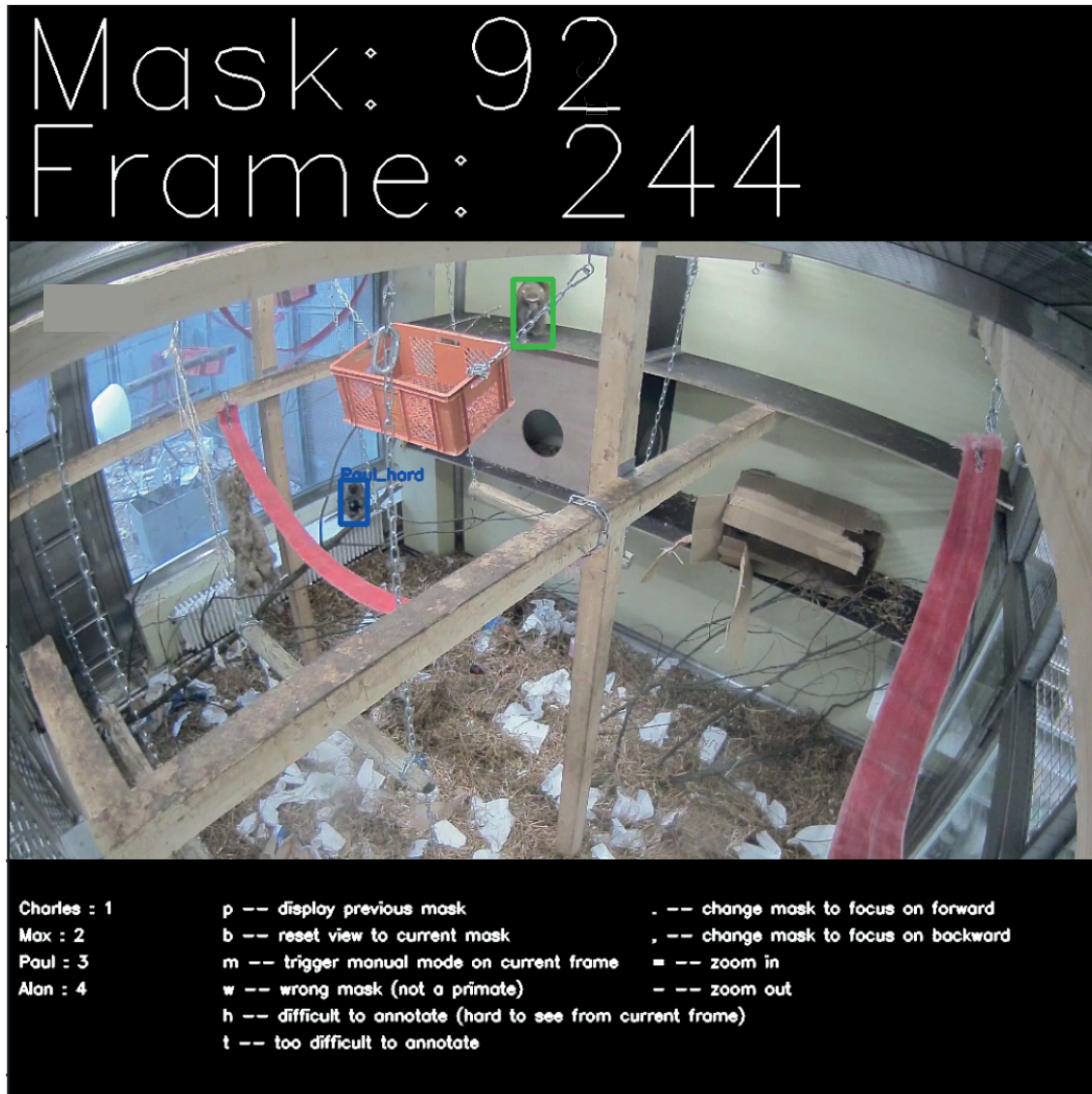
Supplementary Figure 3 | Identification Graphical User Interface. Mask-box results from SIPEC:SegNet is overlaid over frames in blue and can be labeled one by one. The current box to be labeled is in green. A simple keyboard input scheme is provided within the GUI. Names of individuals and the number of masks to be labeled can be set by the user.
