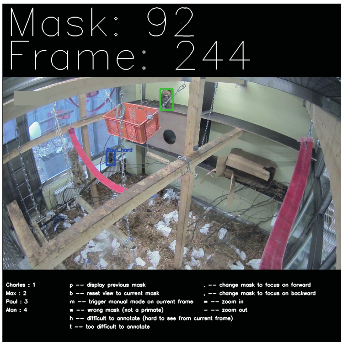
Supplementary Fig. 3 | Identification Graphical User Interface. Mask-box results from SIPEC:SegNet is overlaid over frames in blue and can be labeled one by one. The current box to be labeled is in green. A simple keyboard input scheme is provided within the GUI. Names of individuals and the number of masks to be labeled can be set by the user.
