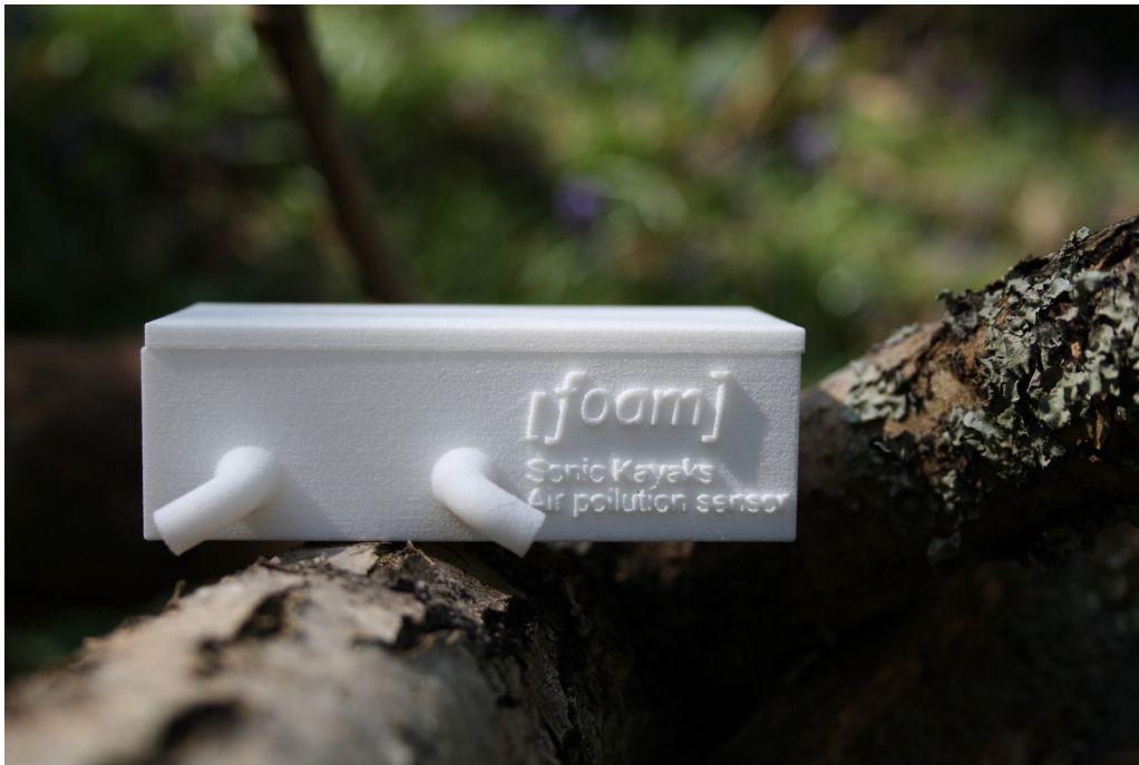
Figure 3. Custom housing for PMS7003 air quality sensor.
