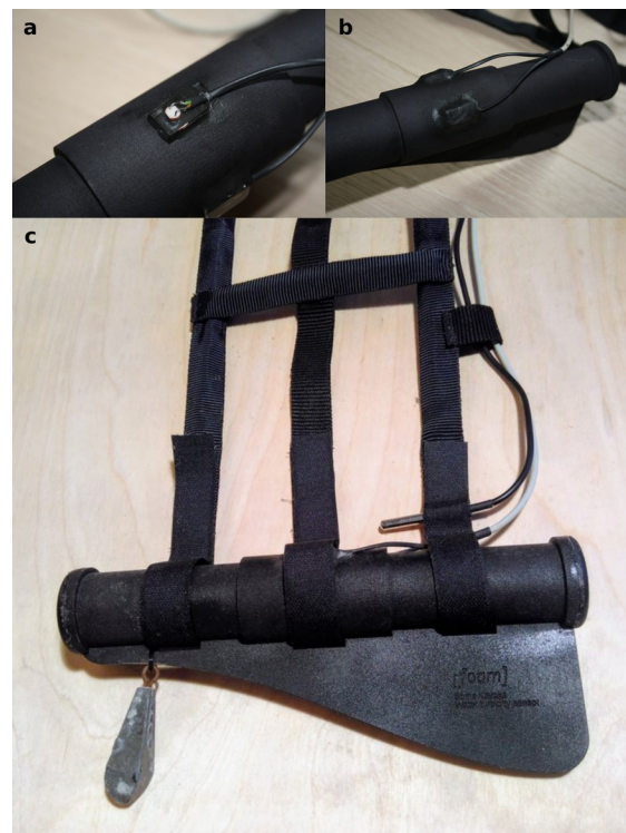
Figure 4. (a) Electrical component (LDR) set in resin block attached to the turbidity tube, (b) Both electrical components (LED and LDR) attached to the turbidity tube and coated to block light, (c) The completed turbidity sensor attached to the nylon rigging with velcro straps, with the temperature sensor just above, and an optional weight.
