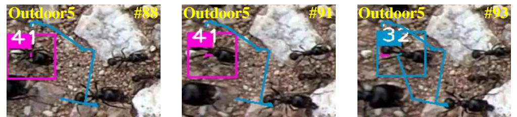
Fig 7. Drift at the scene boundary. A newly-entered Ant No.41 is mis-associated with an existing Trajectory No.32.
