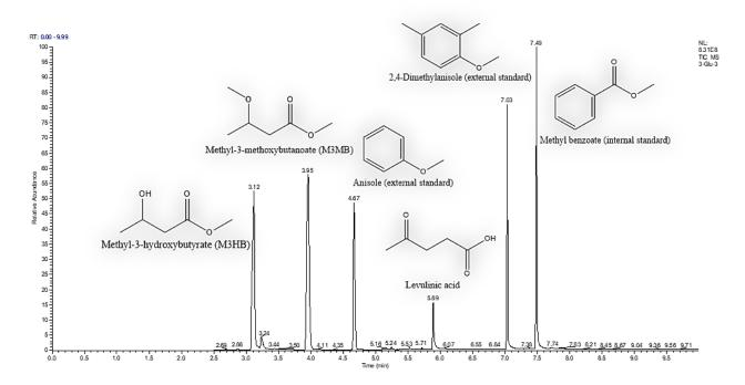
**Figure 5.** GC-MS chromatogram of methylated derivatives of 3HB (M3HB and M3MB), levulinic acid and three standards (anisole, methyl benzoate and 2,4-dimethyl anisole).
