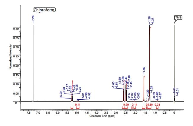
Figure 8. <sup>1</sup>H NMR spectrum of the P(3HBV) produced by *Cobetia* isolate no. 105 when grown on
