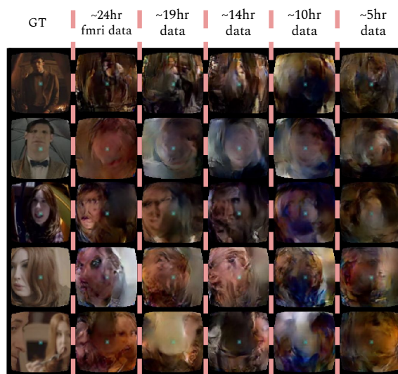
Figure 5. Time experiment: Reconstructions from the brain2pix fixed RF method trained on various amounts of fMRI data after 50 epochs of training. Ground truth (GT), ~24hr is the entire dataset, ~19hr is \frac{4}{5} , ~14hr is \frac{3}{5} , ~10hr is \frac{2}{5} , ~5hr is \frac{1}{5} of the dataset.
