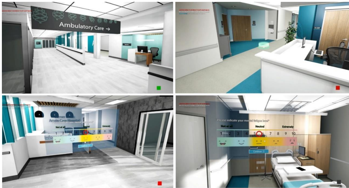
Figure 3. Screenshots from the participants' view in the virtual environment. The bottom two images show our integrated Likert-scale widgets that simplify the collection of subjective feedback. The integrated software platform also helps to keep track of the duration of the wayfinding tasks, the position of the user in the environment, and the times at which the user looks at certain signs or other selected environmental features.
