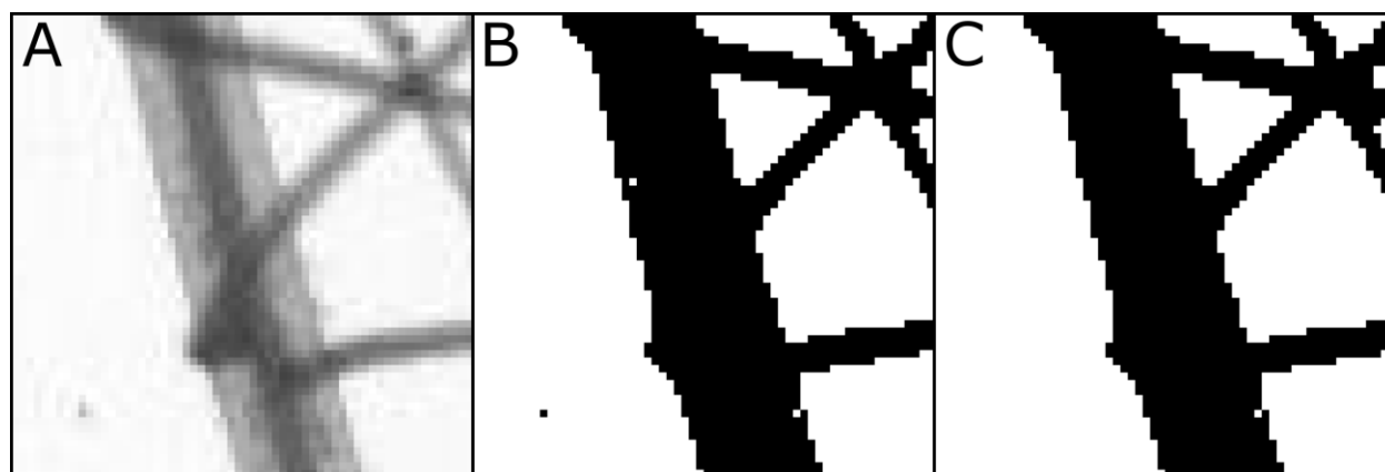
Figure 2. (A) Selected region of a plant root image taken from a flatbed scanner with a transparency unit. (B) Segmented image without noise filtering. We observe that the dark component on the white background is caused due to soil particles and a white component on the root portion is caused due to brighter root texture. (C) Segmented image with noise filtering. The white pixel at the bottom is not considered as a hole because the pixel is only surrounded by seven root pixels, rather than eight.
