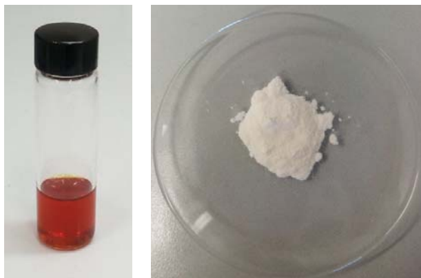
Figure S1. AnchoisOil extracted from anchovy filleting waste ( left ), Omeg@Silica comprised of MCM-41 silica loaded with 50% w/w fish oil ( right ).
