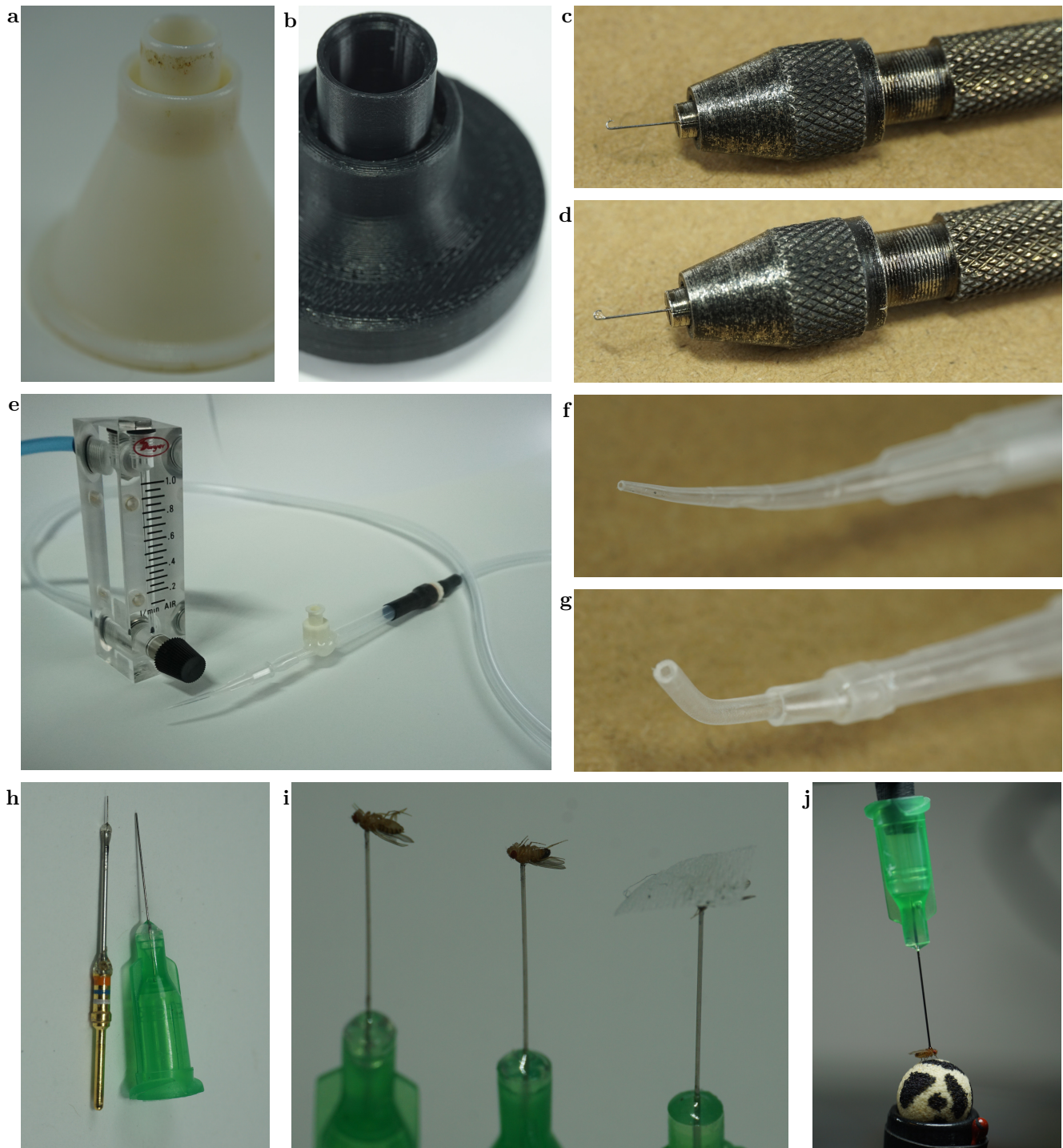
Figure S5. Gallery of useful tools: a, b: 3D-printed funnels used to move flies between bottles and vials. A bent minuten pin used to move the fly in the Sarcophagus and apply glue, without glue c and d with glue. e Flowmeter to regulate negative pressure for the fly picker. Tip of the fly picker made from micropipette tip (f) and shrink tube (g). h Traditionally made tether (left) and blunt dispensing tip with Luer lock alternative (right). i tethered flies in holding area prior to experiments, the 3rd holding a piece of tissue. j Body-fixed, tethered fly on a ball, showing the modest ‘uphill’ orientation of the fly
