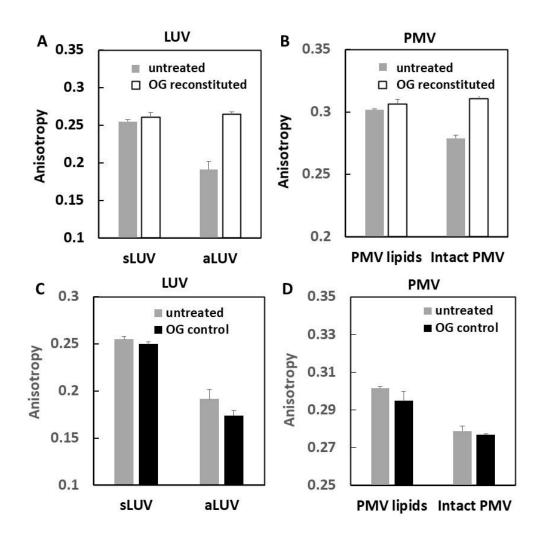
Figure 4 Reconstitution of intact PMV increases membrane order. (A and C) Artificial LUV, (B and D) PMV derived vesicles. Anisotropy of DPH fluorescence was measured at 16°C on: (gray bars) untreated vesicles; (open bars) reconstituted vesicles prepared by dissolving lipid vesicles in 45 mM OG and then diluting to 1.5 mM OG; (black bars) vesicles to which 1.5 mM OG was added as a control (OG control).
