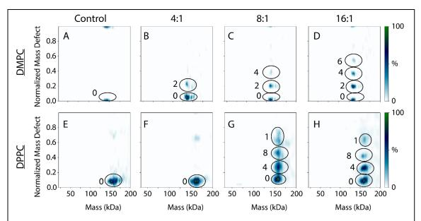
**Figure 6:** Native MS intensities as a function of normalized mass defect versus mass for the WT TM-AM2 in DMPC nanodiscs (A–D) and DPPC nanodiscs (E–H), with no TM-AM2 added (A, E), a 4:1 ratio (B, F), an 8:1 ratio (C, G), and a 16:1 ratio of TM-AM2 to nanodisc.
