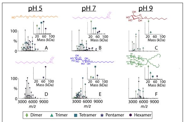
**Figure 2**. Representative native mass spectra with the deconvolved mass spectra in the inset of AM2 (at  $50 \mu M$  per monomer) solubilized in (A) C8E4 at pH 5, (B) LDAO at pH 7, (C) OG at pH 9, (D) LDAO at pH 5, (E) DDM at pH 7, and (F) LMNG at pH 9. Each detergent is shown above the spectrum. Average oligomeric state distributions collected in triplicate are shown in Figure S1.
