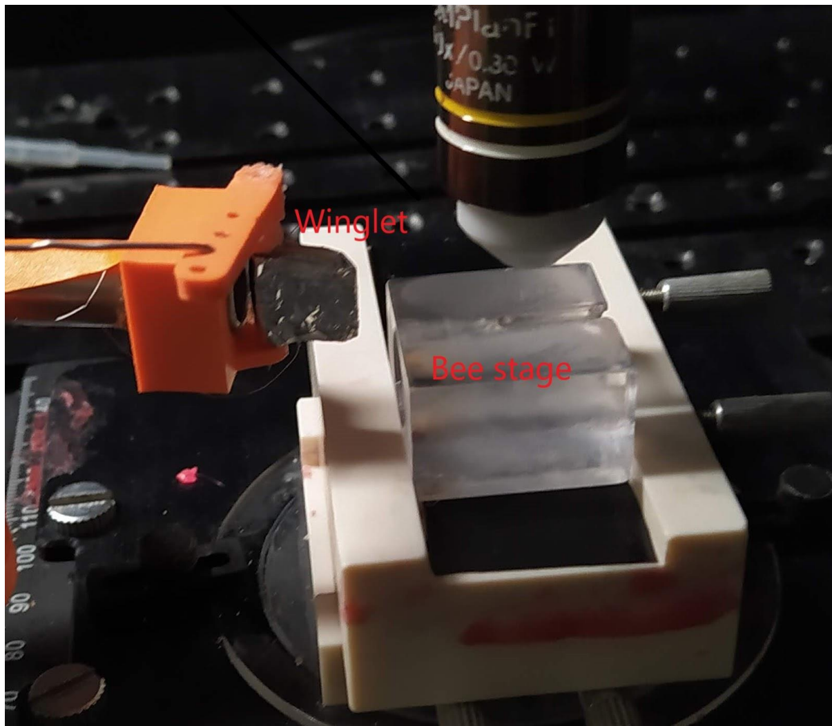
Fig. 5 Stimuli generator. Bees are mounted on the stage facing the winglet. The airflow is directed through the steel tube straight toward the antennae. The winglet is activated by a motor whose speed is detected through a rotary encoder.
