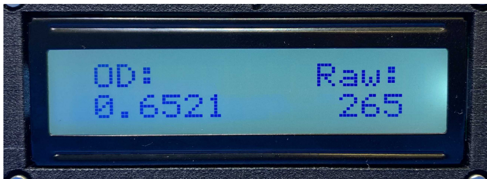
Figure 10: Device screen in OD mode, showing OD and raw intensity values.
