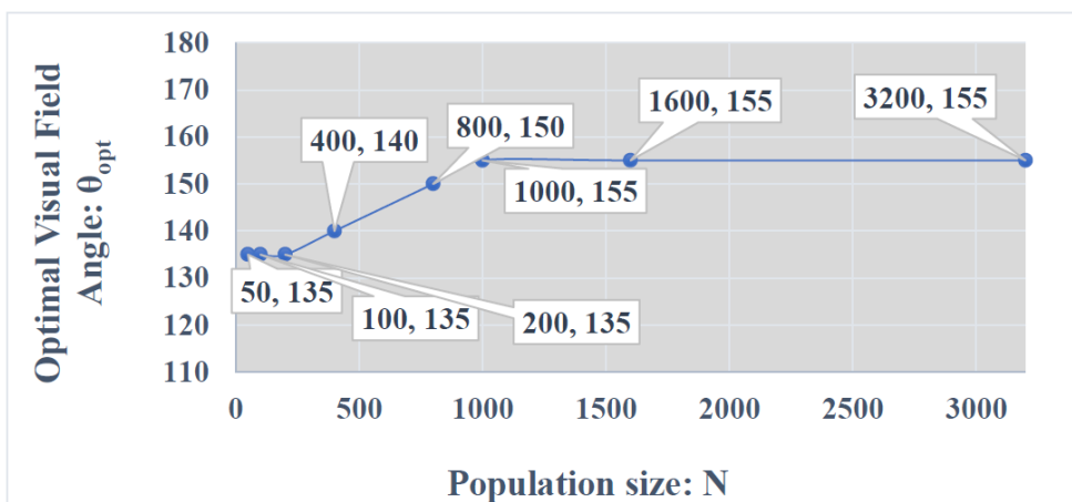
Figure 10: The best view angle changes with the population size. (The system conducted 100 experiments under different field of view of each population size, and global order P of each experiment corresponds to an average over 1000 simulation time steps following a 10000 time step pre-equilibration period.)
