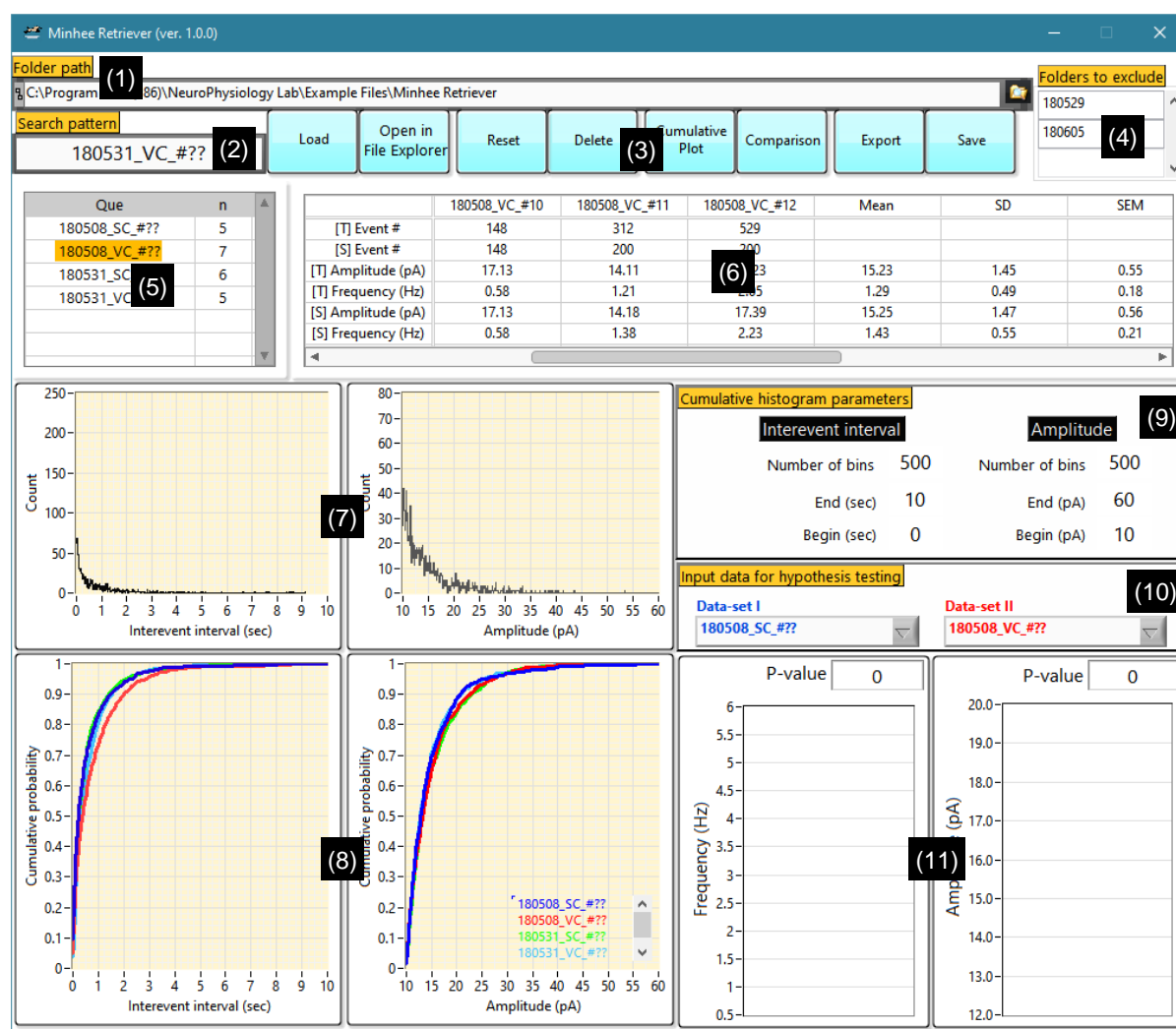
Figure 7. Screen capture of Minhee Retriever's GUI. The GUI of the program has 11 subsections (numbers in parentheses). (1) The Folder Path is used to specify the top-level folder that contains the unit file. (2) A user can enter search patterns to retrieve unit files. (3) Several Action buttons are available to execute the functions. (4) The unit files listed here are excluded the during retrieval. (5) Query table. This table shows currently retrieved results. (6) The result table shows the number of events, amplitude, and frequency of the total and selected events in each unit file. General (7) and cumulative relative (8) histograms for the IEI and amplitude of selected events. (9) Parameters for generating the cumulative relative histogram. (10) For statistical comparison between two groups, two data-sets are determined by a user. Result of hypothesis testing is displayed in (11).
