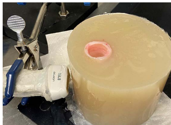
Figure 2: Imaging phantom constructed from ex vivo porcine trachea encased in agar.
