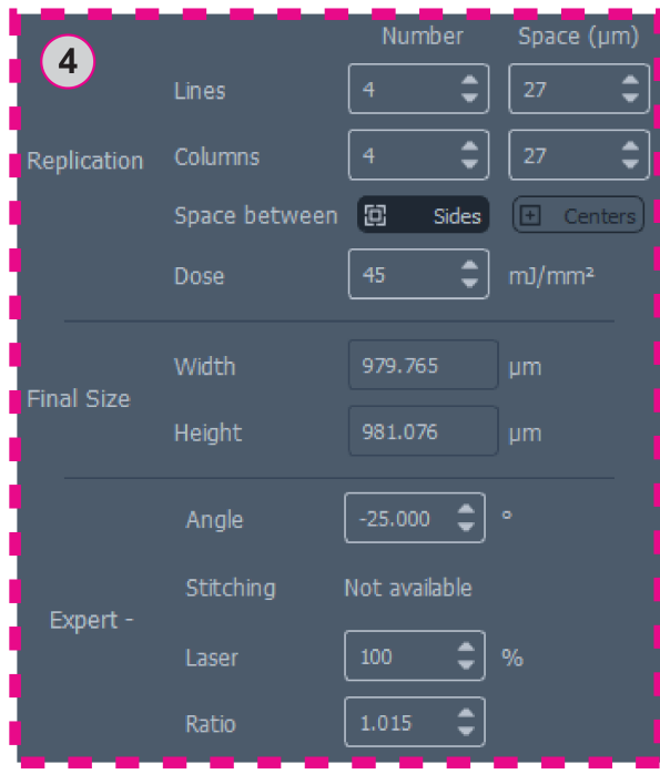
627 Figure 2. Screen shot of Leonardo software with pattern positioned on grid. Area 1 contains 628 the \mu\text{m}/\text{pix} ratio for pattern design. Area 2 is the ruler for measuring your grid. Area 3 is where 629 to add or change patterns and ROIs. Area 4 contains all of the information for pattern 630 positioning and dose. Area 5 contains options for patterns including toggling overlays, copying 631 or deleting patterns, and selecting patterns for micropatterning. Area 6 is where templates can 632 be saved and loaded. Larger views of areas 4 and 5 are shown below for clarity. 633
