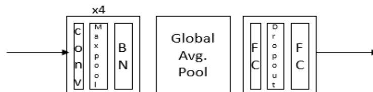
Figure 3. Architecture of the 3D Convolutional Neural Network (CNN).
